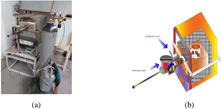
Fig. 3. Torrefaction unit for pre-treatment of pine waste (a– Improved Joule heating system, b– Technical drawing of heating system)
