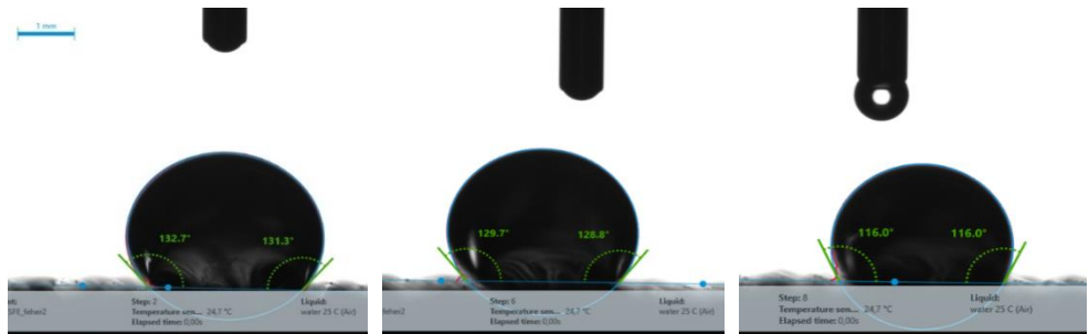
Fig. 21. Photograph of a water drop residing on FDM 3D-printed PLA surface during the measurement using the Eos method, for three tests at identical conditions
