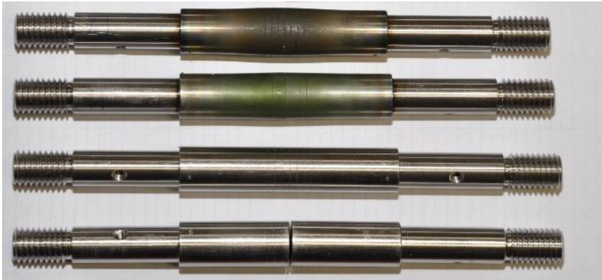
Figure 3. The Gleeble specimens RG3 (reference experiment), DG3 (diffusion bonding specimen) with the same heat and axial load, below the initial pieces
