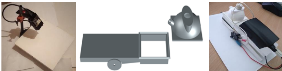
Figure 1. – Picture of designed prototypes, left the measuring stand, middle the model of the measuring head, right the improved model
