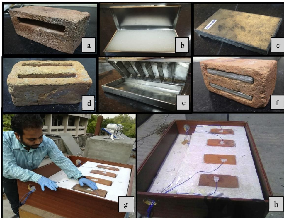
Fig. 2.17. Fabricating steps of PCM-incorporated bricks; (a) Single-slot brick, (b) Encapsulation container, (c) Macroencapsulated PCM, (d) Double-slot brick, (e) Encapsulation container with fins, (f) PCM-incorporated brick with twin slots, (g) Installation of bricks and (h) Final setup (Saxena et al., 2020)
