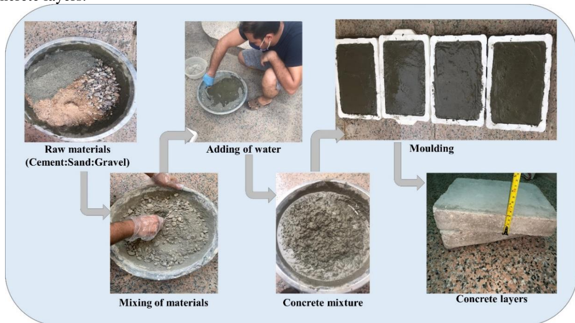
Fig. 3.5. Fabrication procedure of concrete layers
