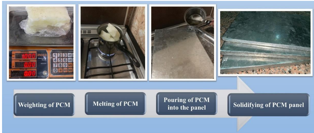
Fig. 3.10. Preparation procedure of PCM panels
