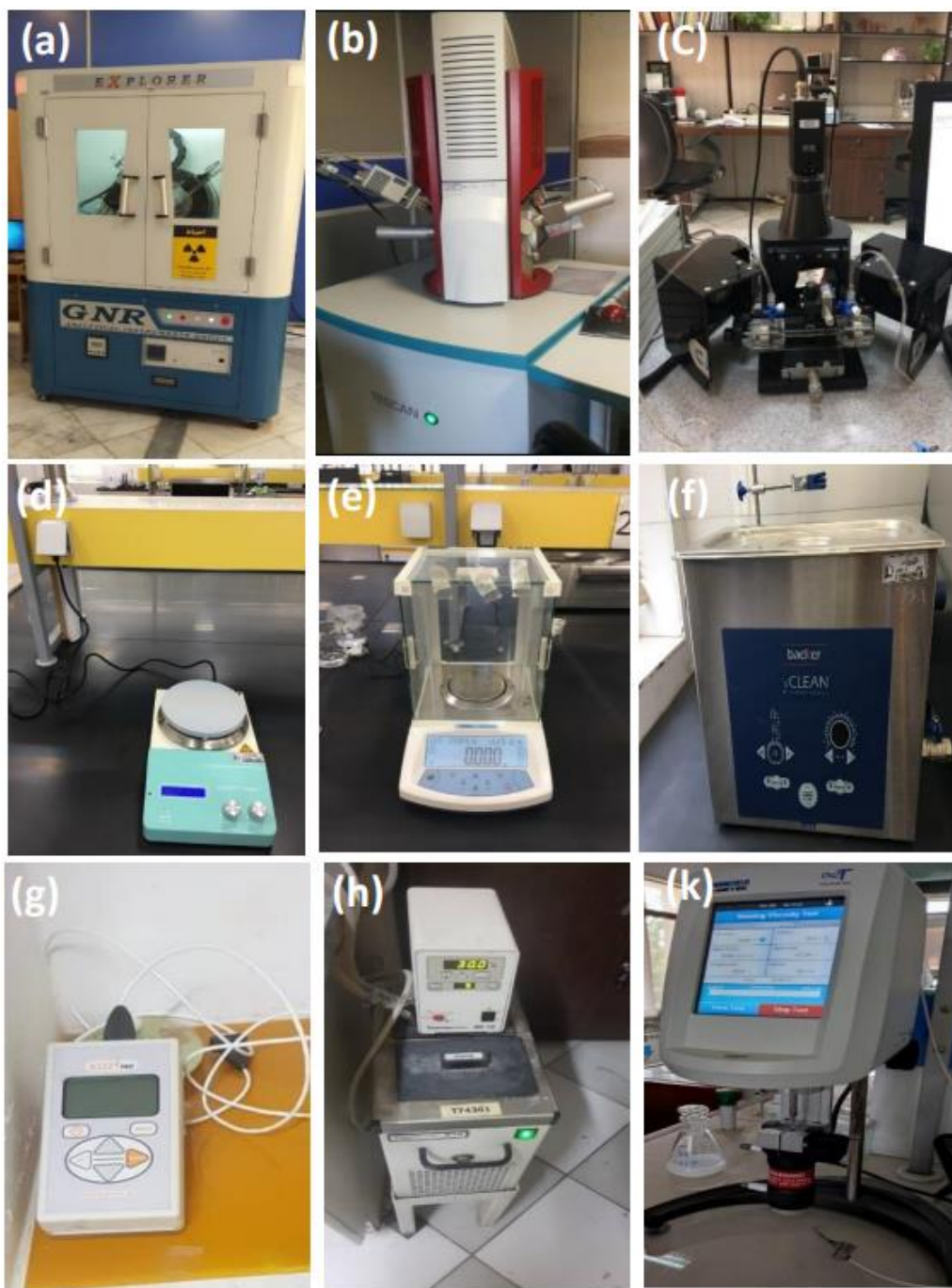
Fig. 3.2. Laboratory devices: (a) XRD, (b) FESEM, (c) Zeta potential analyser (d) Magnetic-stirrers, (e) Digital scale, (f) Ultrasonic, (g and h) KD2-Pro plus temperature control, and (k) Rotational viscometer
