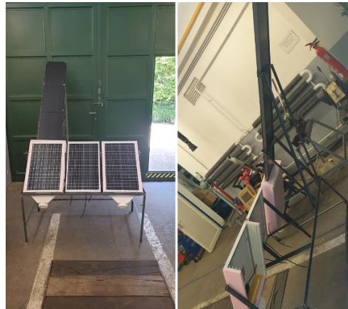
Fig. 5. The PV/T duct and PV modules are installed on the supporting iron structure.
