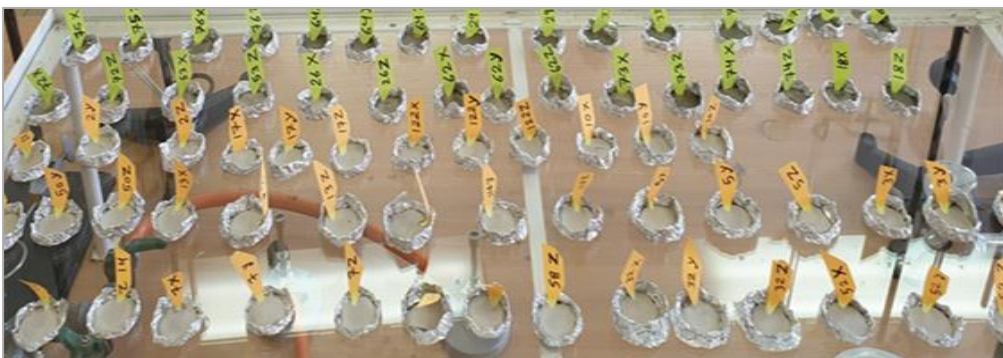
Figure2. Mortar-incorporated adsorbed ash composite
