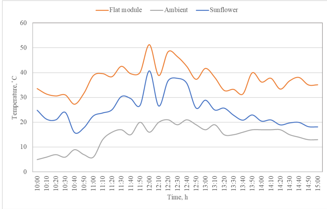
Fig. 4.13. PV systems temperature measurement ( \alpha=30^\circ )
