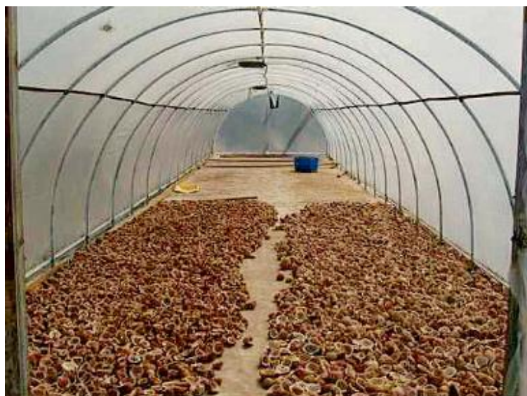
Fig. 2.10. Direct solar drying for food drying, India (Eswara & Ramakrishnarao, 2013)
