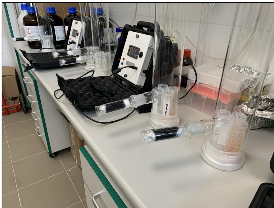
Figure 9. Picture of the open-loop-pull-type DHS sampling system during the competitive binding site investigation, as described in Section 4.2.4
