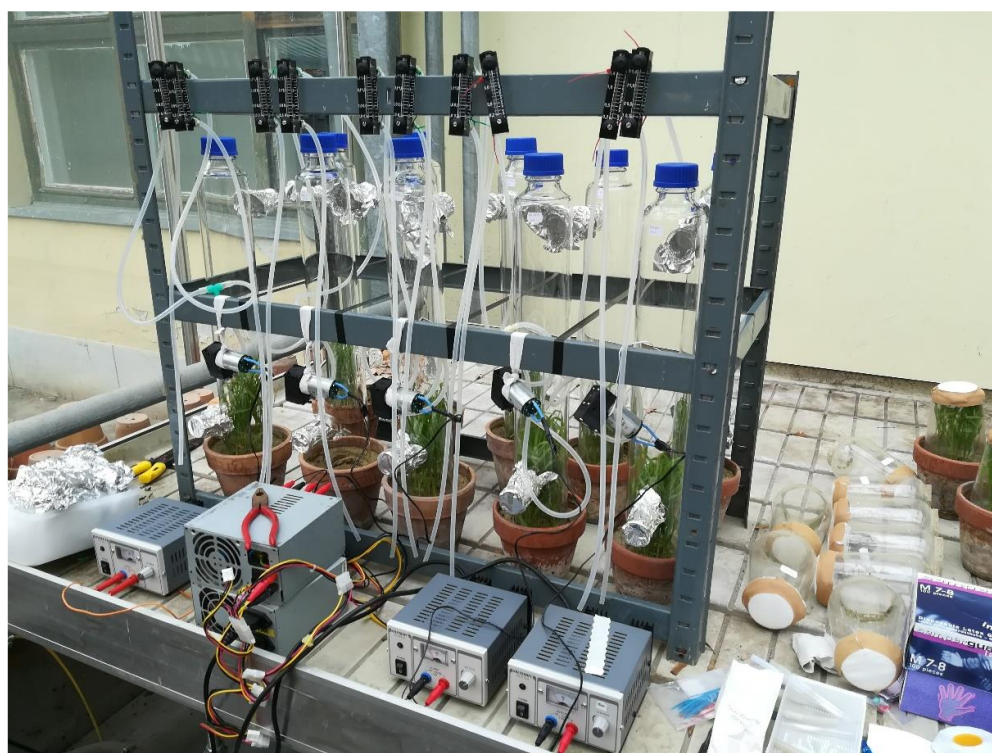
Figure 10. Sampling setup for DHS sampling consisting of eight pots of wheat plants and two blank pots under glass cups with air in- and outlets located in the bottom and the top
