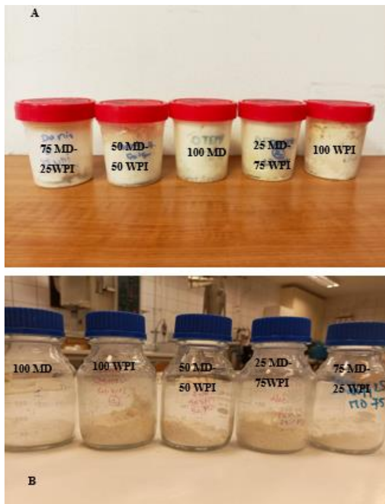
Appendix- Figure 5: Picture of oil loaded dried microcapsules obtained by different drying methods. A: microcapsules obtained by freeze-drying, B: Microcapsules obtained by spray-drying.
