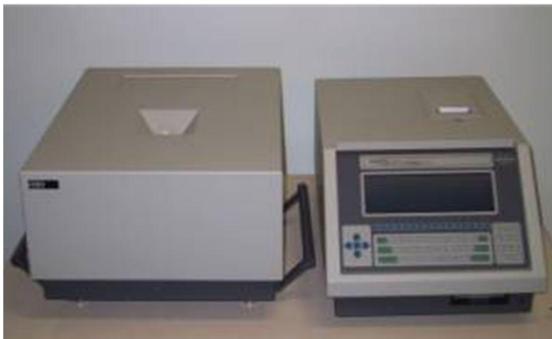
Figure 4. 2 Nuclear Magnetic Resonance spectrometer (NMR) Bruker pc 120 Minispec
