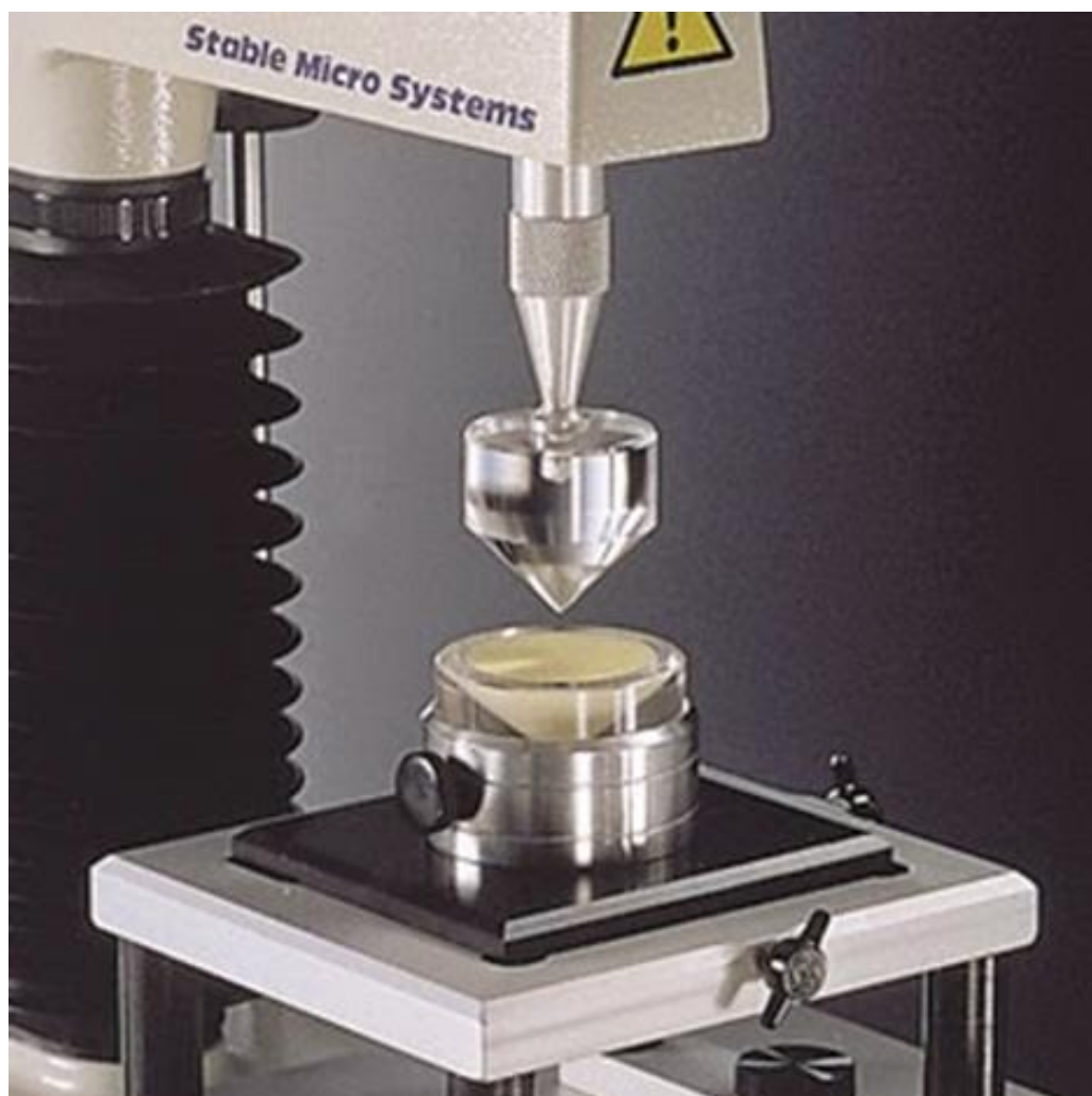
Figure 4. 6 Texture analyser (TA-TX Plus, Stable Micro System, UK)
