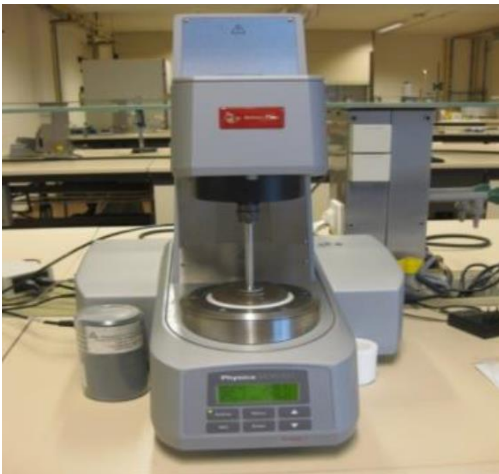
Figure 4. 7 Rheometer (MCR 301, Physica/Anton Paar, Ostfildern Germany–Europe)
