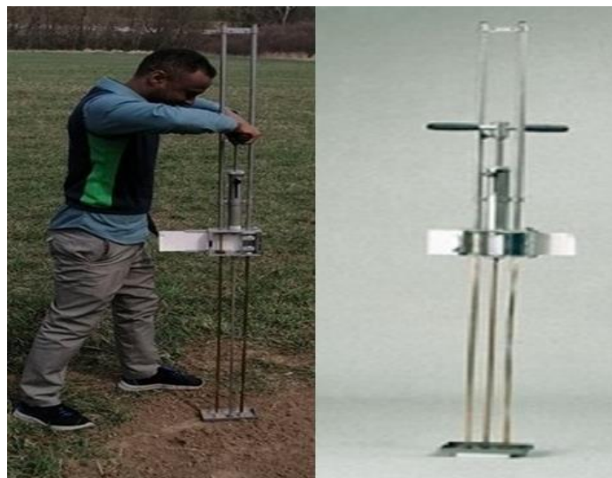
Figure 3.5. Cone penetrometer (06.02 Penetrograph) while the measurement.
