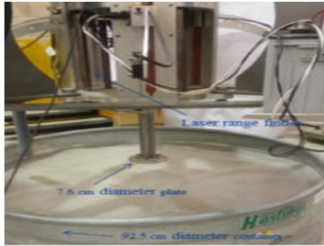
Figure 2.11. Normal bevameter test set up (Michael B. Edwards et al., 2017).
