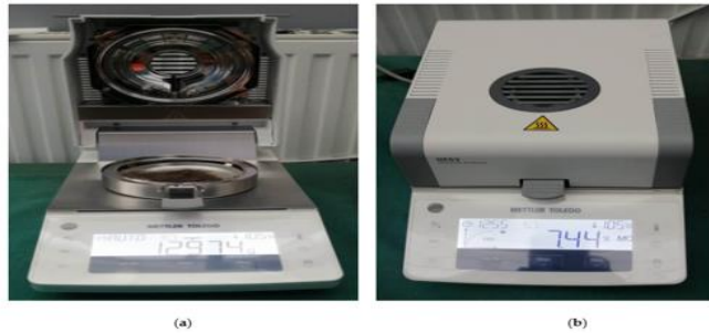
Figure 2.3. The analyzer (a) shows the mass sample, and (b) shows the percentage of the moisture content.
