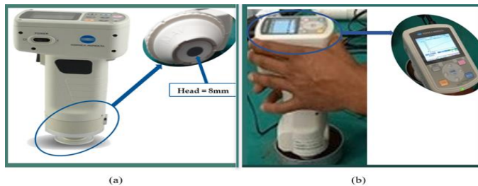
Figure 2.4. Shows (a) the Spectrophotometer (CM-700d) and the 8mm head (the electromagnetic waves pass through), and (b) while measuring and recording the data.
