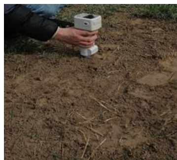
Fig. 6.5. Soil spot prepared, and the spectrophotometer usage in field.
