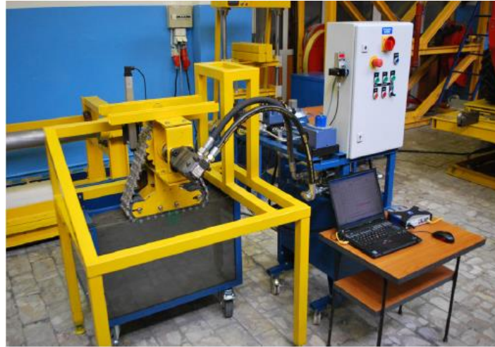
Fig. 3.20. The new device used for measuring quasi-static and dynamic shearing strength of the soil (Dudzinski and Damian, 2019).
