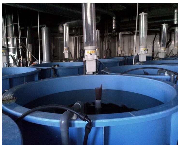
Figure 3.1. Recirculating aquaculture system (RAS) used for fish feeding trials
