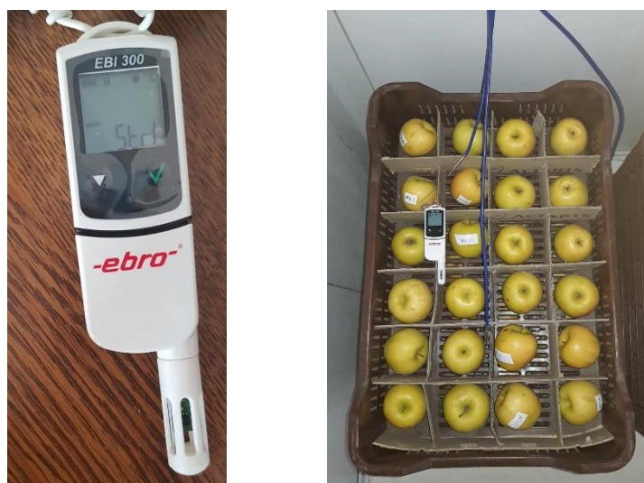
Fig. 3.2. The Ebro EBI 300 TH Multi-Use USB Data Logger for temperature and humidity measurement
