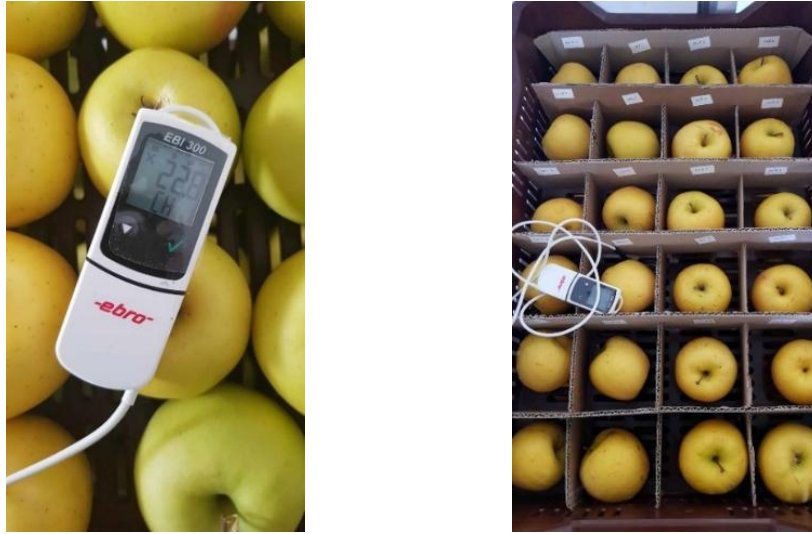
Fig. 3.1. The Ebro EBI 300 TE multi-use USB datalogger with external temperature probe
