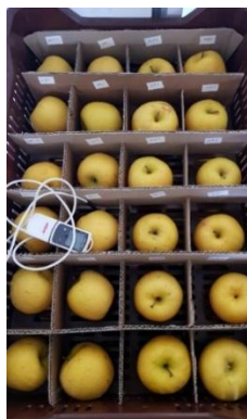
Fig. 1. The Ebro EBI 300 TE multi-use USB datalogger with external temperature probe
