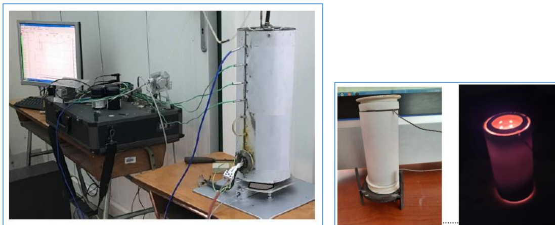
Figure 6. Directly electrically heated, air-inlet laboratory reactor, maximum operating temperature: 1300 °C (MATE lab)
