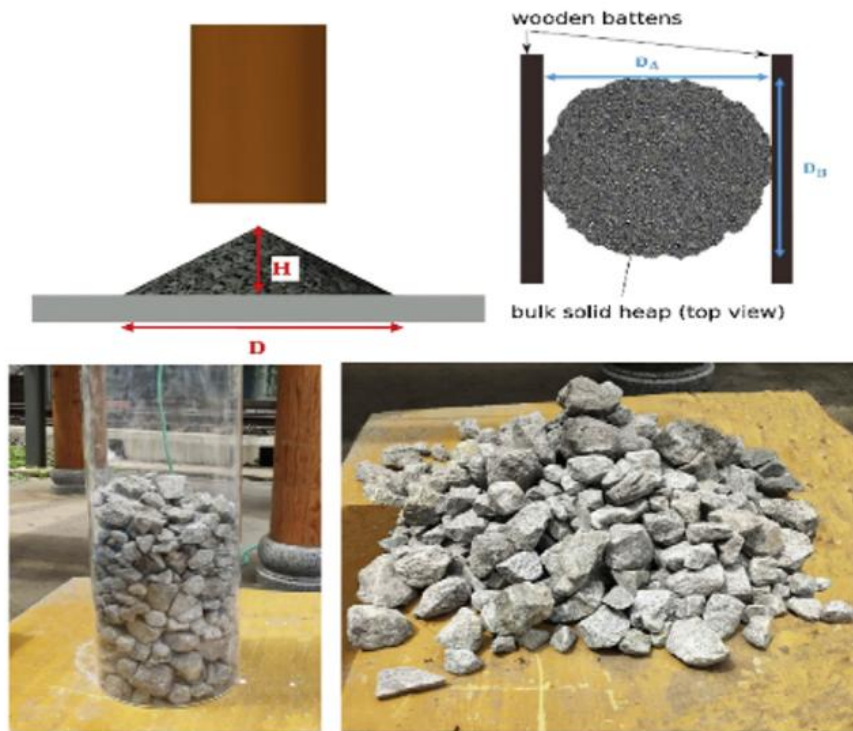
Fig.2.35. Photos of the angle of repose test (Aela et al., 2022).
