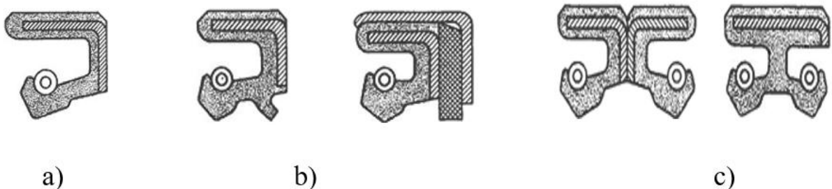
Fig.2.11. Shows several sealing: a) single seal, b) auxiliary sealing lip, and c) double seal (Neale, 1995).
