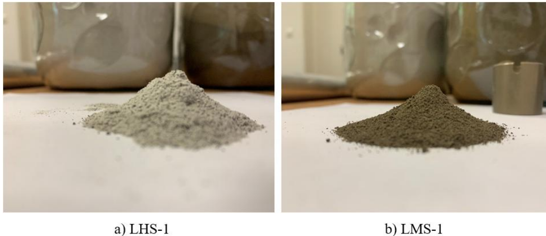
Fig.3.10. Angle of repose test example photos
