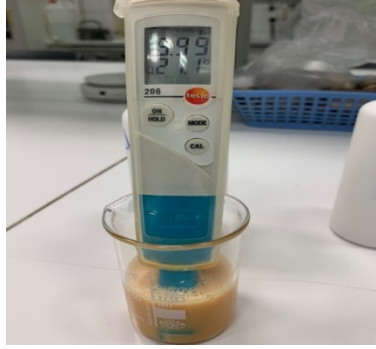
Figure 5: pH measurement for liquid whole eggs using a portable pH (Testo 206; Testo-AG, Germany)
