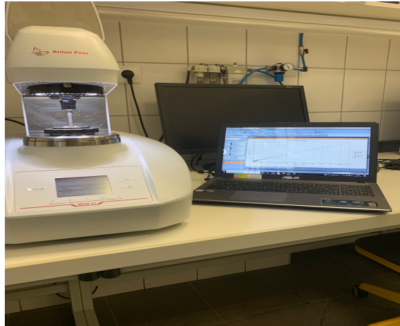
Figure 7: Measurements of rheological properties of liquid egg products samples with a rotational rheometer using MCR 92 rheometer (Anton Paar, Les Ulis, France).
