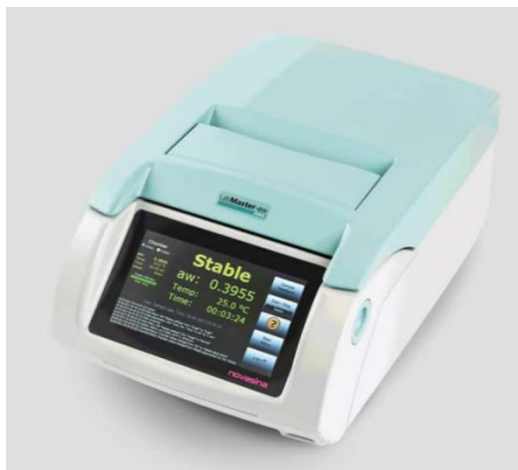
Figure 8. Water activity equipment (LabMaster-aw neo) used for the experiment (Image source: Internet 1)
