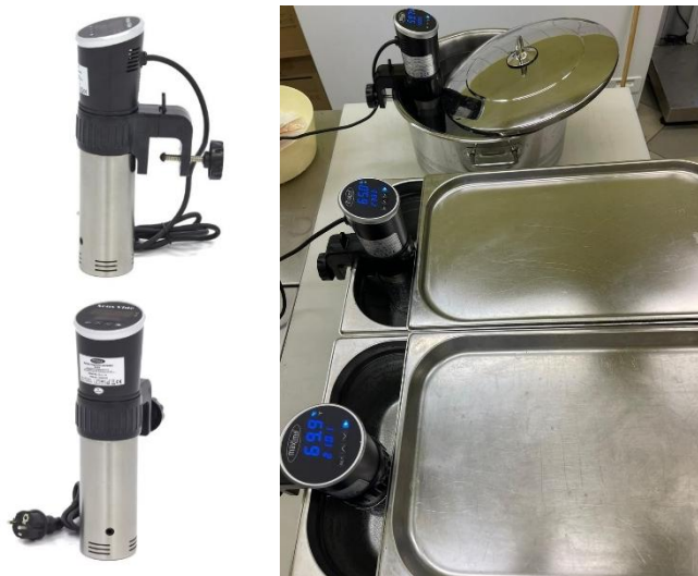
Figure 7. Sous-vide equipment (Maxima) used for the experiment and treatment of vacuum-packed wild red deer meat samples during sous-vide processing (Photo by author)
