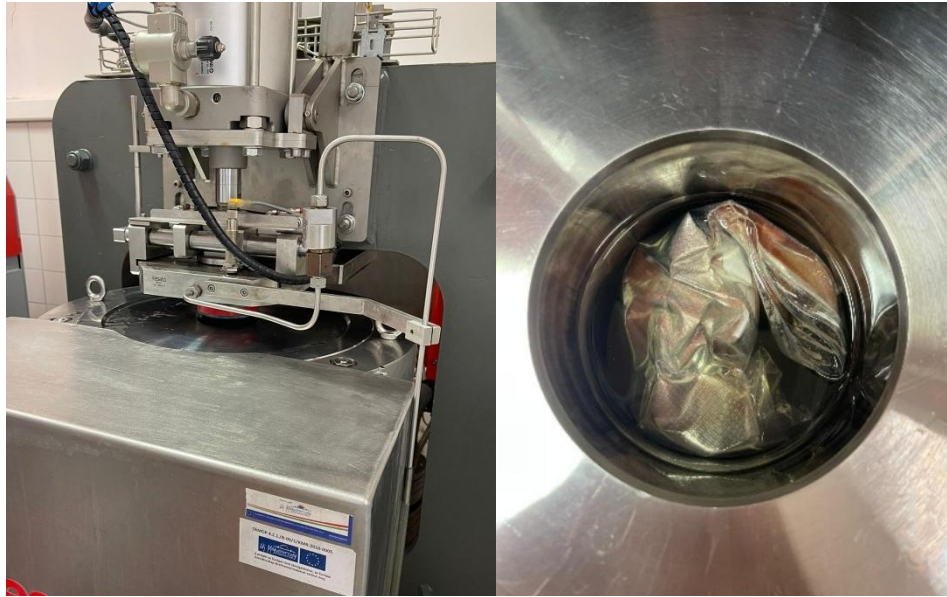
Figure 6. Resato FPU-100-2000 HHP equipment and loaded vacuum-packed meat samples into the HHP chamber. (Photo by the author)
