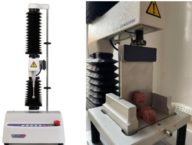
Figure 10. TA.XT Plus Texture Analyzer (Stable Micro Systems) used for the measurement and the measurement process during the texture analysis of wild red deer samples (Photo by the author)
